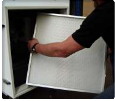
Pre & secondary filter holding frame
